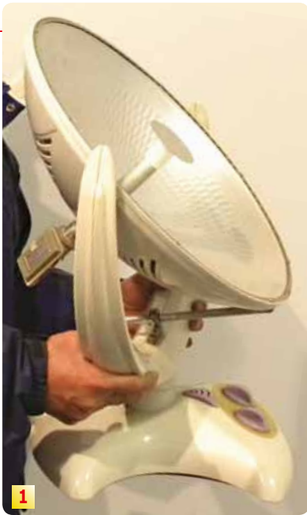
1. Another Wenbi Wong creation: a satellite dish made from an out-of-service electric heater. The Cassegrain principle is also very helpful here in finding an elegant solution for the LNB.
