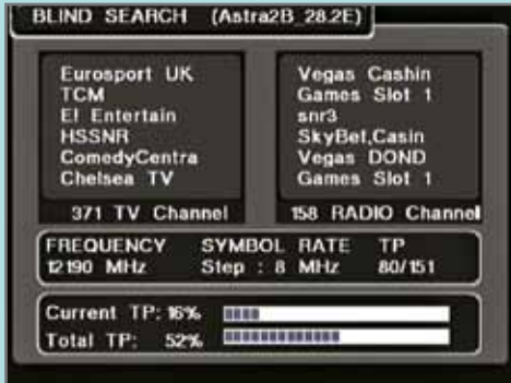
The Blind Scan feature can find transponders that are not already in the preprogrammed list |
