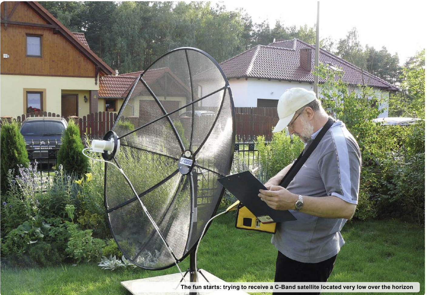
Time to align the antenna. We recommend to use a water level equipped with an angle meter – it will make setting the elevation much easier.
