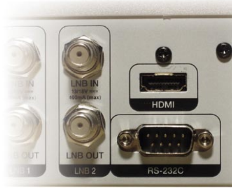
The decisive HDMI port which Eycos uses to output the scaler signals
