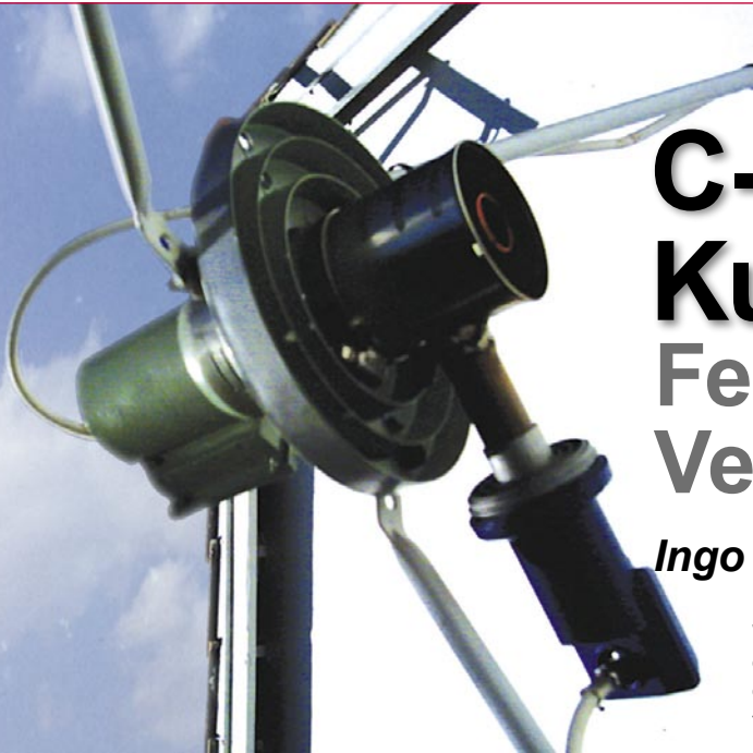
The C/Ku-Band feed used in real life at a 1.80 m dish receiving PAS4 on 72East
