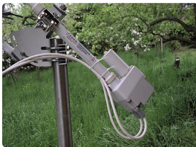
This drive motor moves the antenna support
