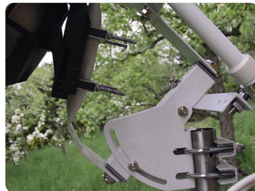
The latitude scale is used to align the dish according to the geographic latitude of the location
